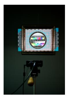
► First of all, take advantage of this test pattern to focus your projector. In our case we have to turn the ring around the lens of the Acer projector.
